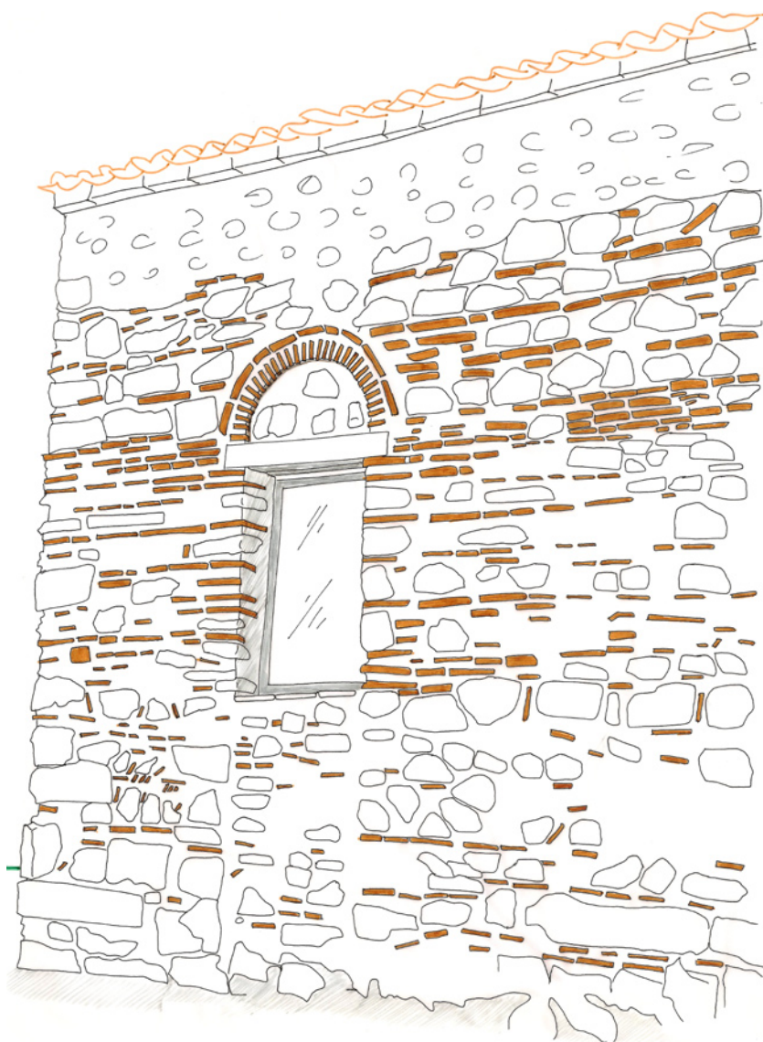
Fig. 72. Panagia Peninsula near Vonitsa, Panagia Monastery, katholikon. A) The original masonry in the NE corner and the N half of the apse. B) Drawing of a section of masonry in the E part of the N façade.
